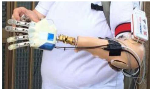
Fig. 7. The prosthetic hand containing sensors and electrodes which allow to “feel” in real-time the shape, roughness and consistency of grasped objects.
