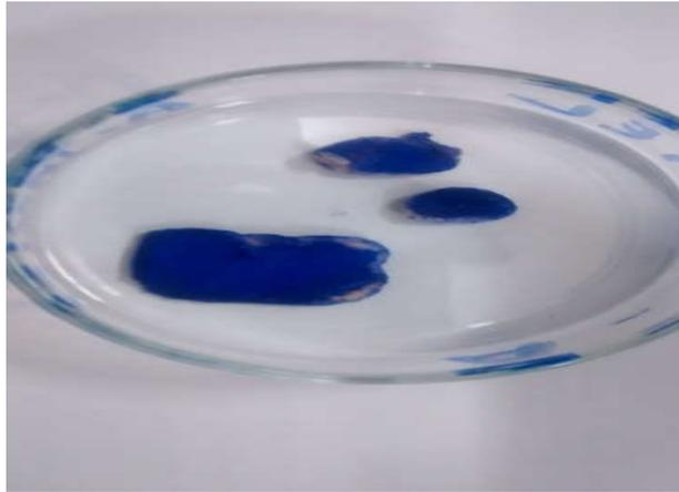
Figure 6 Methyl blue dye absorbed nano cellulose fiber aerogel
