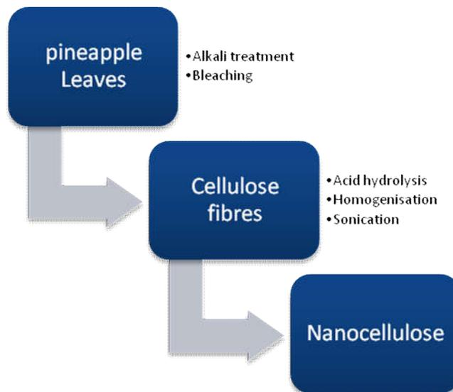
Figure 2 Extraction of CNF
