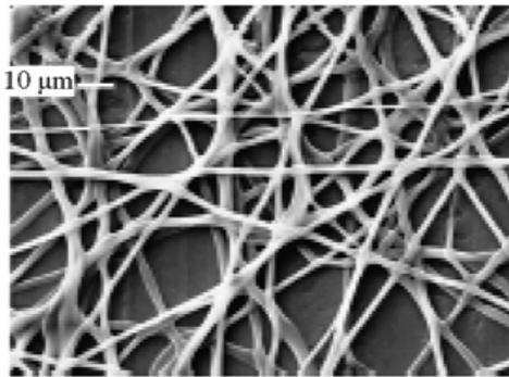
Figure 8 SEM image of CNF aerogel 10  $\mu\text{m}$
