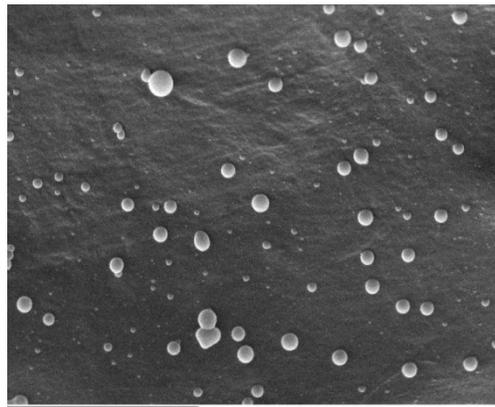
Figure 9 SEM image of silane treated CNF aerogel 50  $\mu\text{m}$
