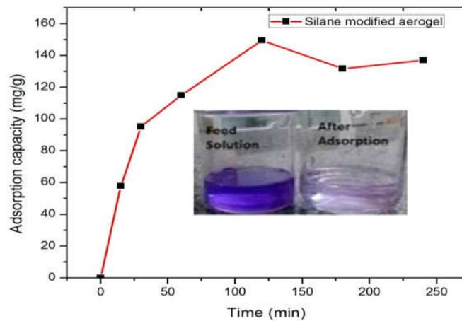
Figure 7 Adsorption capacity vs time graph for silane modified CNF aerogel
