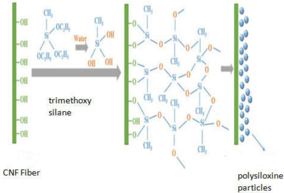
Figure 4 Chemistry of silination
