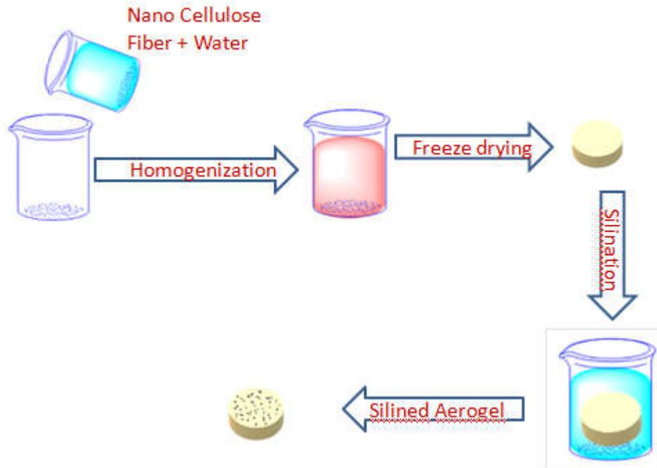
Figure 3 Silination of CNF aerogel
