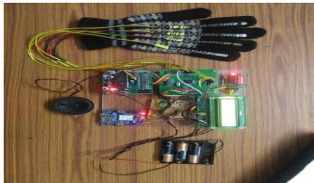
**Fig 4: Sensor part of the system with processing unit, Audio playback module and GSM module**
