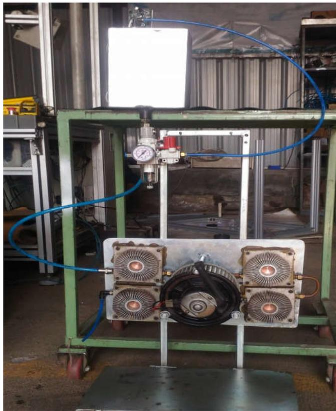
**Figure 1. Experimental set up of Hydraulic Oil Cooler**
