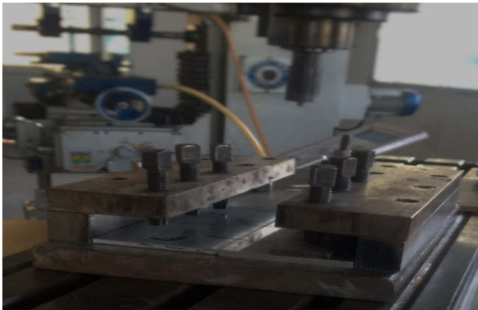
Fig.4 Work piece is mounted in the fixture
