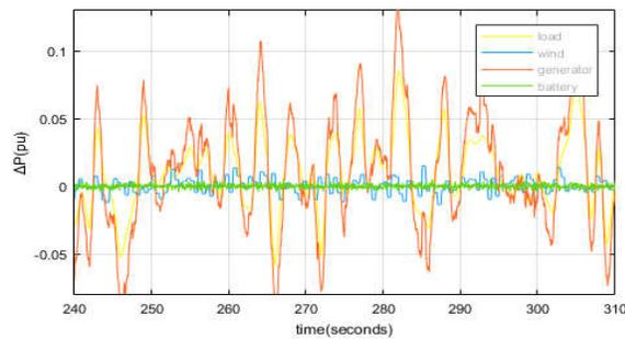
Fig. 13. Power variations with maximum battery power
