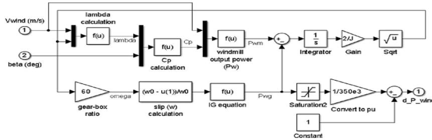
Fig. 4. Wind turbine generator model
