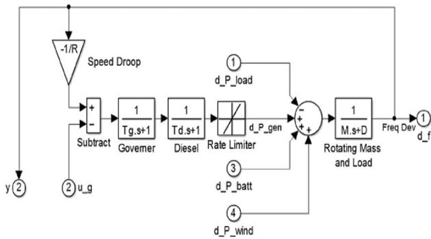
Fig.2. Conventional generator (Small Power System) model
