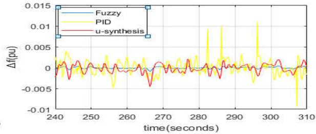
Fig. 16. Frequency deviations comparison between  $\mu$ -syntheses, Fuzzy with full battery attached.
