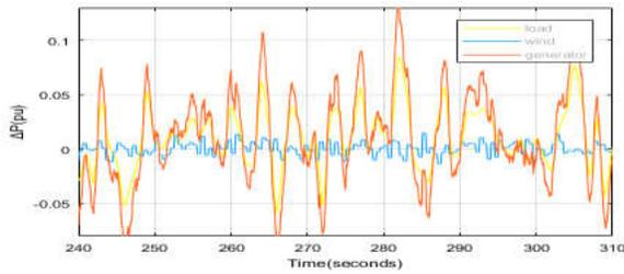
Fig. 15. Power variation without attached battery
