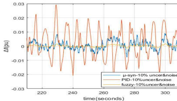
Fig. 18. Frequency deviations comparison between  $\mu$ -syntheses, fuzzy, PID with 10% model uncertainty and measurement noise
