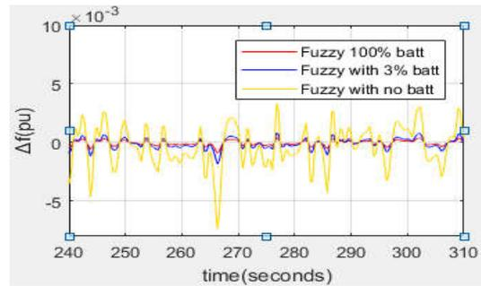
Fig.14.Frequency deviation comparison with fully battery
