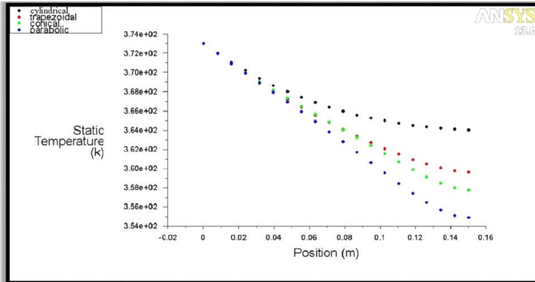
Figure 4.2: CFD Analysis Temperature Plot - Aluminium - Natural Convection Table 5.1:
