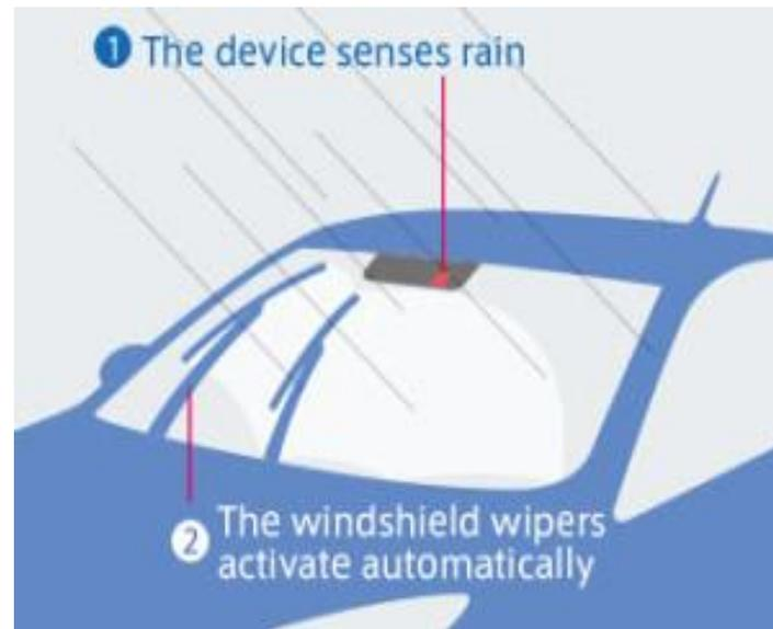
**Fig. 4. Embedded rain-sensing system**
