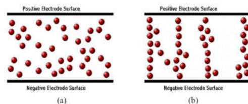
Fig-2(a) ER fluid structure without applied Electric field
