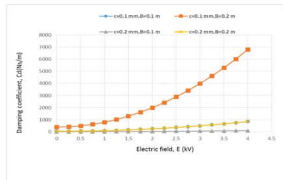
Fig7: Dependency of Damping co-efficient ( $C_d$ ) with Electric field (E)
