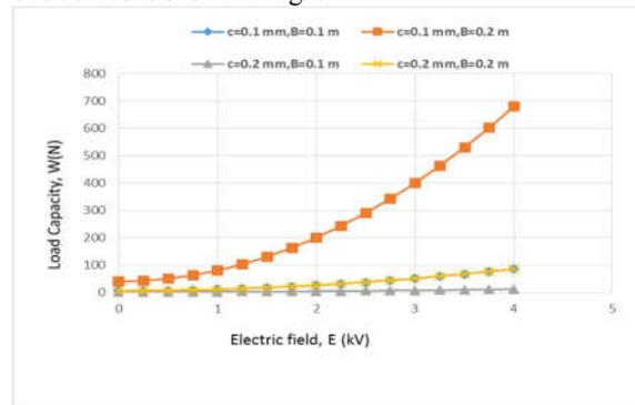
**Fig 5 Dependency of Load capacity (W) with Electric field (E)**
