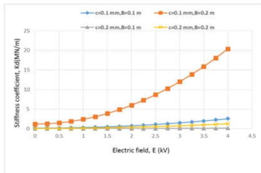
Fig6: Dependency of Stiffness co-efficient ( $K_d$ ) with Electric field (E)
