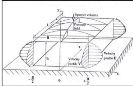
Fig. 3 Squeeze film between two parallel plates
