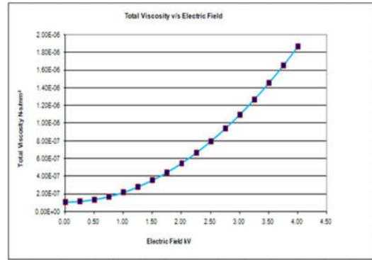
**Fig.4. Dependency of total viscosity with electric field**
