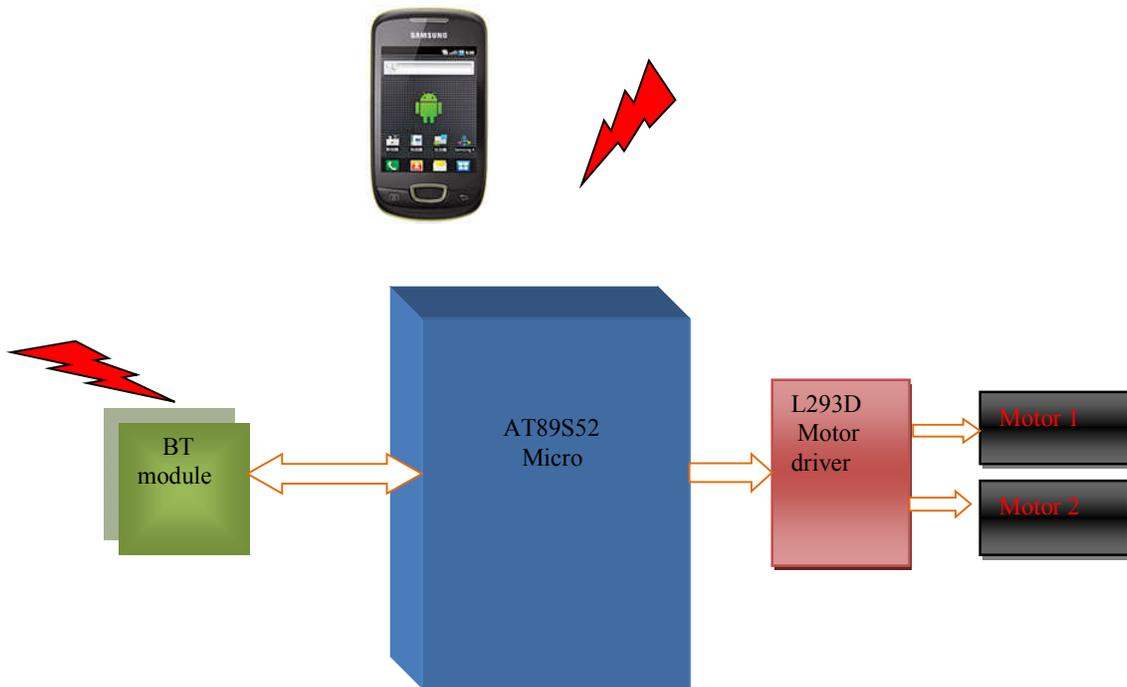
Figure2. Circuit Diagram for Bluetooth module
