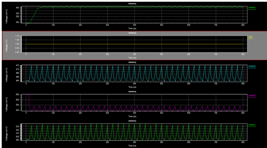
Figure 8. MTCMOS SRAM Cell array simulation
