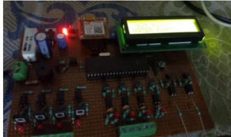
Figure-GSM module and Microcontroller Hardware
