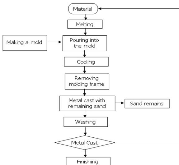
Fig. no. 1.5 Flow chart of casting process
