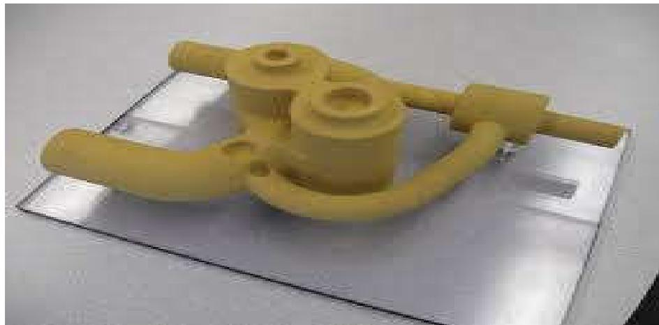
Fig no. 1.7 Core used in casting
