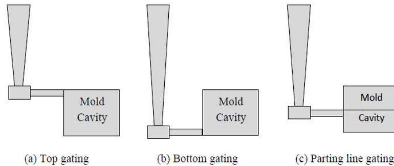
Figure. 1.13 c) Classification of gating system based on parting plane orientation.
