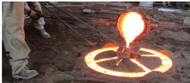
Fig. no. 1.9 Melting and pouring process
