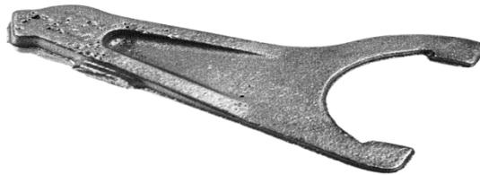
Fig. no. 1.14 Defects due to poor gating
