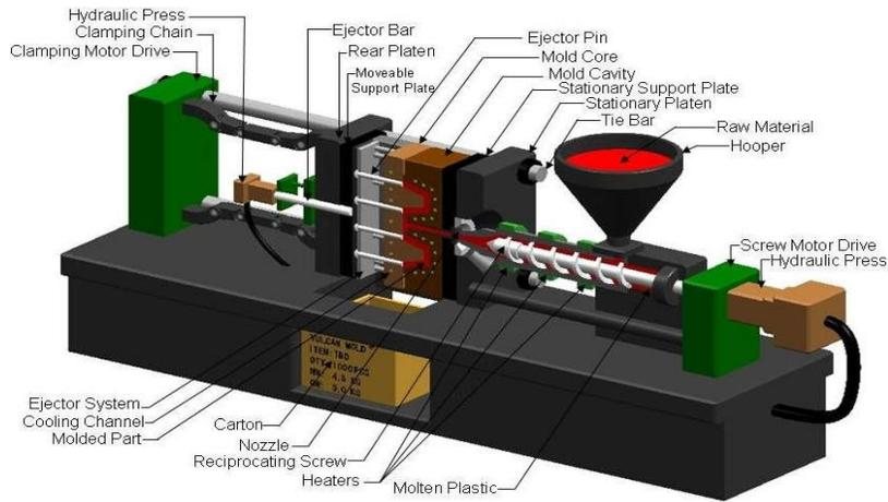
Fig. no. 1.8 Injection molding process
