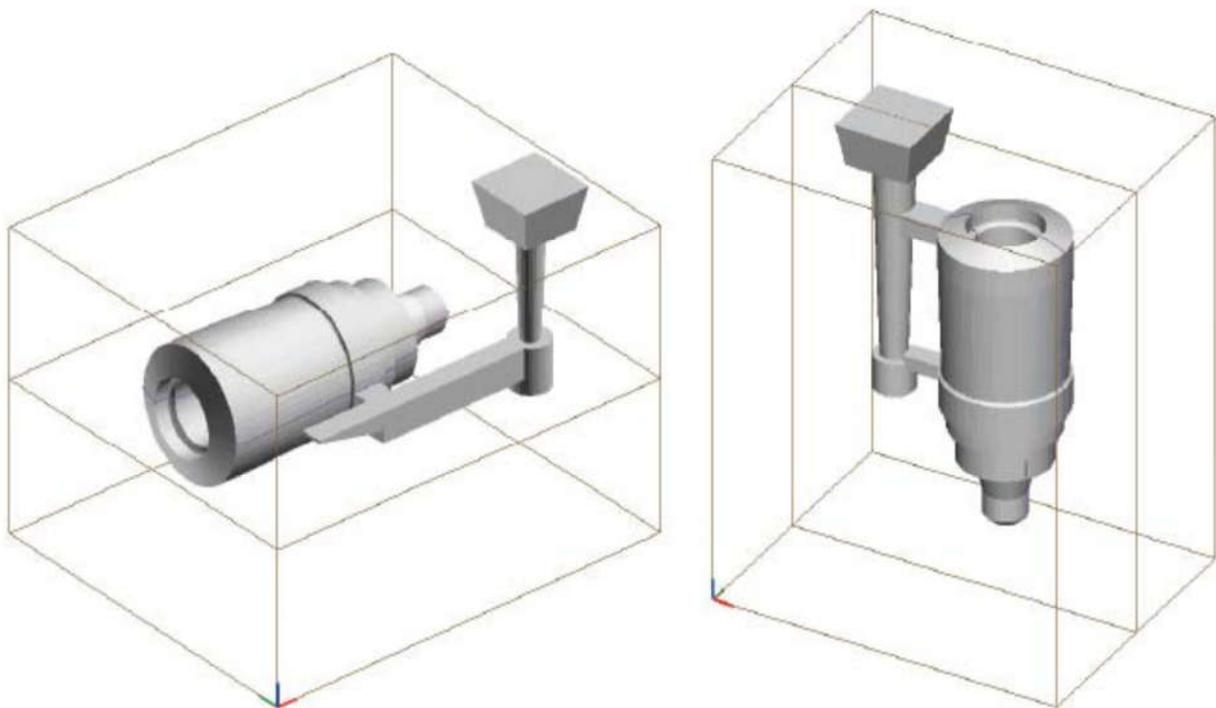
Figure. 1.13 a) and b) Classification of gating system based on parting plane orientation.
