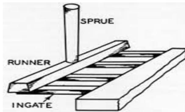
Figure. 1.13 Classification of gating system based on parting plane orientation. (d) Step gate
