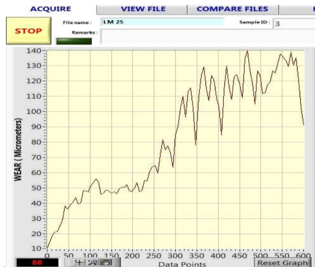
Figure 4. Minimum wear rate 88 µm
