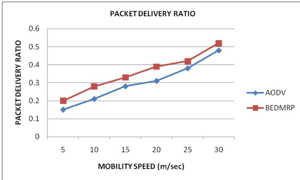
**Fig 1. Packet Delivery Ratio Vs Mobility Speed**
