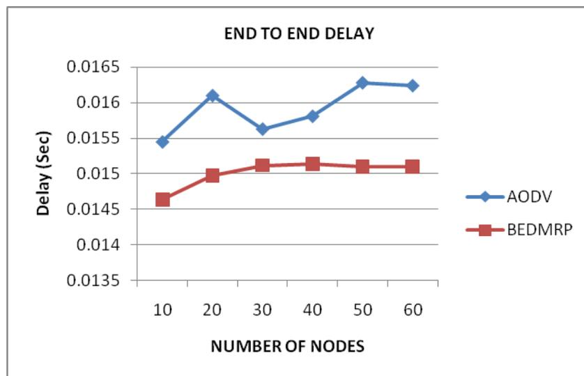
**Fig 2. Delay Vs Number of Nodes**
