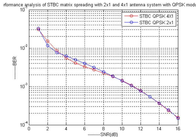
Figure.2.1 BER for STBC permutation for QPSK signaling for 4 transmit antennas, and 2 transmit antennas
