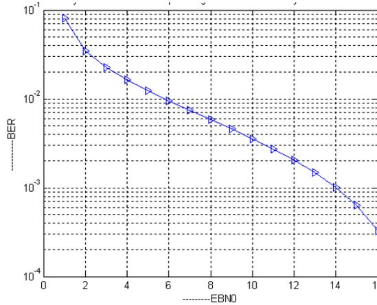
Fig.2 Performance analysis of MIMO-CDMA system employing permutation spreading based on STBC code while considering random channel path gains for 2x1 antenna system with BPSK modulation
