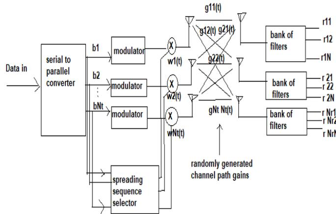
**Figure. 1. Block diagram of MIMO-CDMA system employing permutation spreading with channel path gains**
