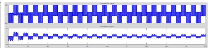
Fig : single phase full bridge inverter voltage and current
