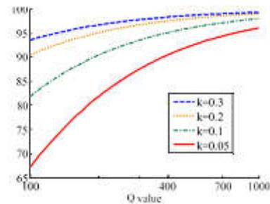
Fig.. Theoretical maximum transfer efficiency between two coils.
