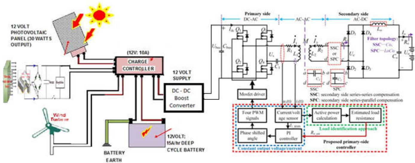
Besides the frequency, the coupling coefficient  $k$  is significantly affected by the design of the magnetic couplers, which is considered one of the most paramount factors in a WPT system. With homogeneous dimensions and materials, different coupler geometry and configuration will have a paramount difference of coupling coefficient. A better coupler design may lead to a 50%–100% amelioration compared with some non optimal designs.
