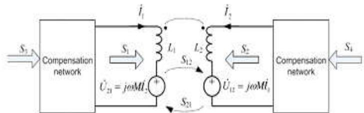
Fig. General two-coil WPT system.
