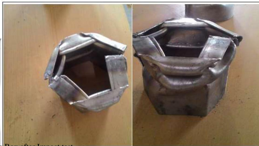
Fig -6: Hexagonal Crash Box after Impact test
