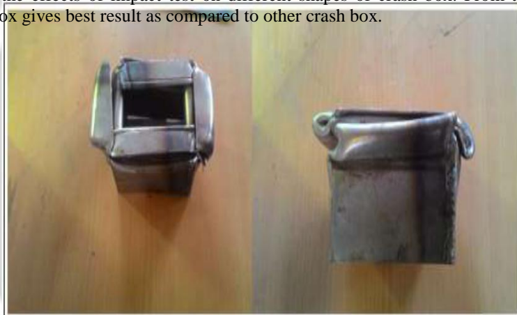
Fig -2: Different Shapes of Crash Box before Impact test
