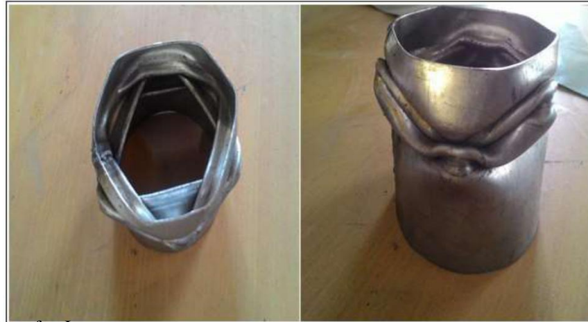
Fig -5: Circular Crash Box after Impact test
