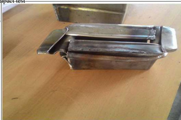
Fig -4: Rectangular Crash Box after Impact test
