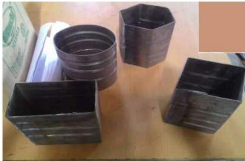
Fig -2: Different Shapes of Crash Box before Impact test
