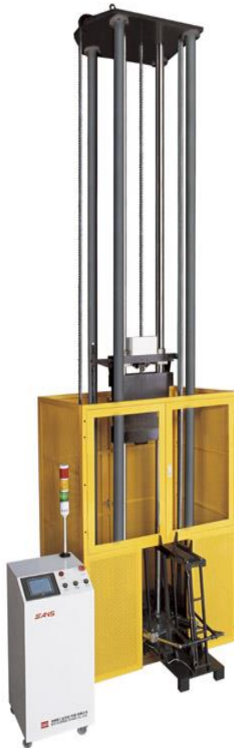
Fig -1: The impact test setup
