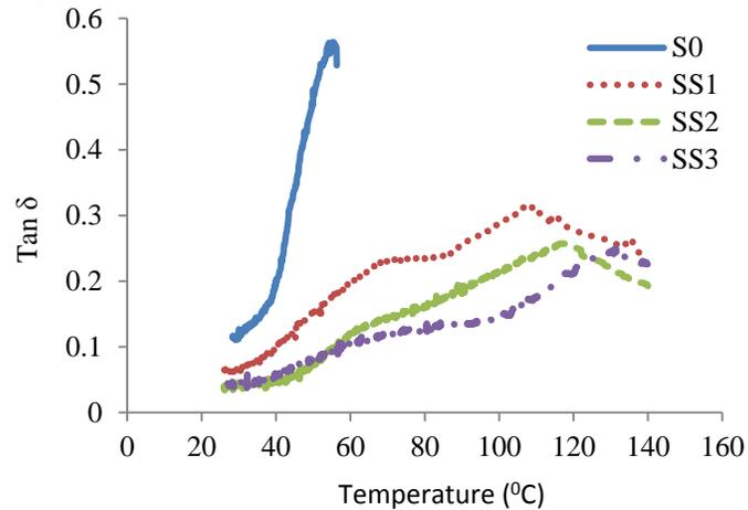
Fig. 3.3: Graphical representation of  $\tan\delta$  as a function of temperature for sugarcane fiber biocomposites
