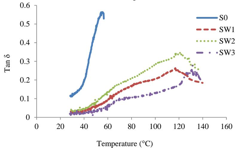
Fig. 3.4: Graphical representation of  $\tan\delta$  as a function of temperature for wheat straw fiber biocomposites
