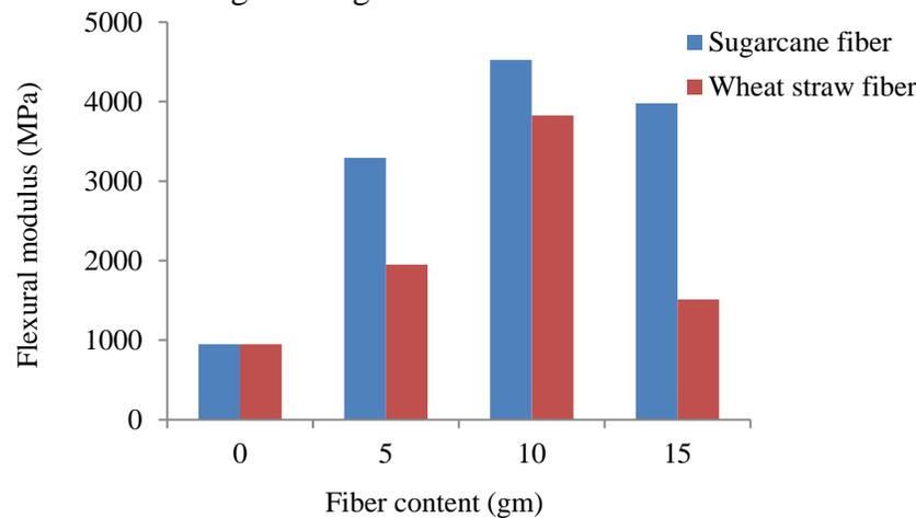
Fig. 3.2: Flexural modulus of sugarcane fiber and wheat straw fiber biocomposites
