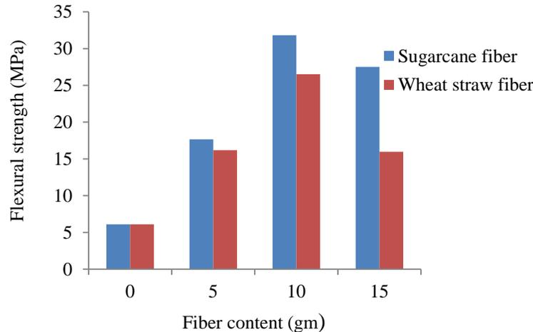
Fig. 3.1: Flexural strength of sugarcane fiber and wheat straw fiber biocomposites
