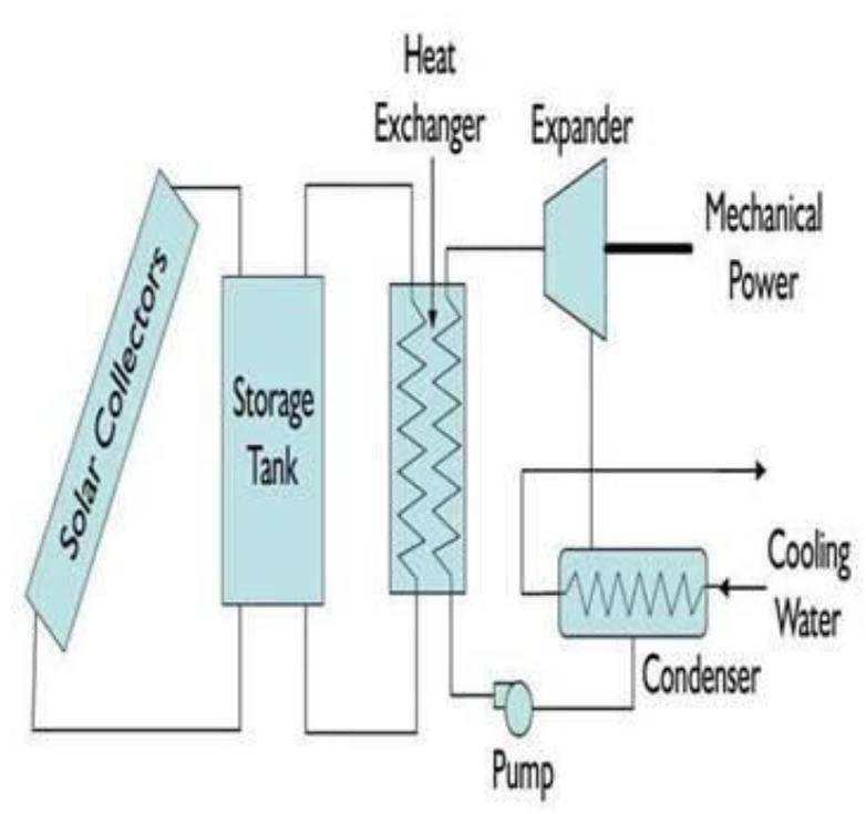
200°C. Both intensity of solar radiation as well as difference of temperature between entering fluid and ambient govern the efficiency of solar collector. The efficiency of such a system is lower than solar electric method using non-concentrating PV modules. Solar Mechanical is advantageous only when solar trackers are used but, the use of such systems is limited to large refrigeration systems only i.e. at least 1000 tons.
