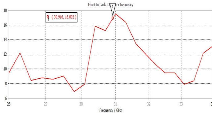
**Figure 11. Simulated Front-to-Back Ratio.**
