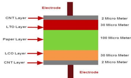
**Fig.2.1.Paper battery Structure**
