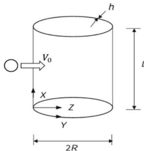
**Figure 1.** The geometry and coordinate system of a carbonnanotube-reinforced composite (CNTRC) cylindrical shell
