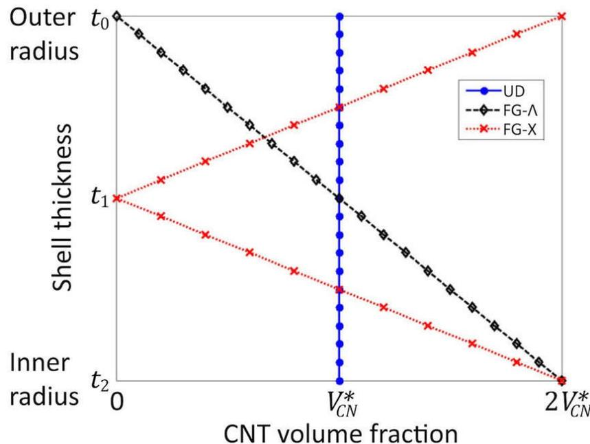
Figure 2. The variation in CNT volume distribution across the shell thickness for the uniformly distributed (UD) and functionally graded CNTRC shells.
