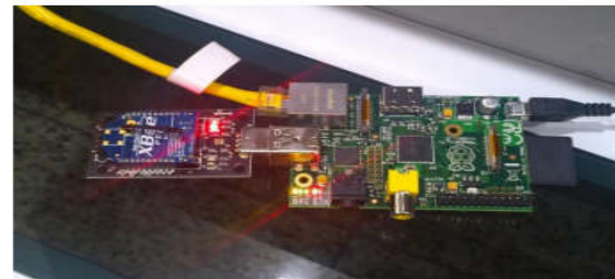
Fig: 12. Interfacing between raspberry pi
