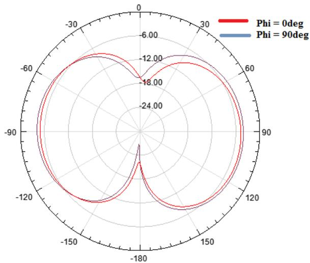
Fig. 4 Radiation pattern at 2.41GHz
