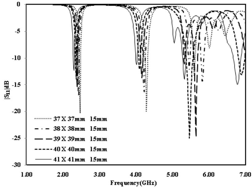
Fig 3: Return loss of antenna for variation in ground plane
