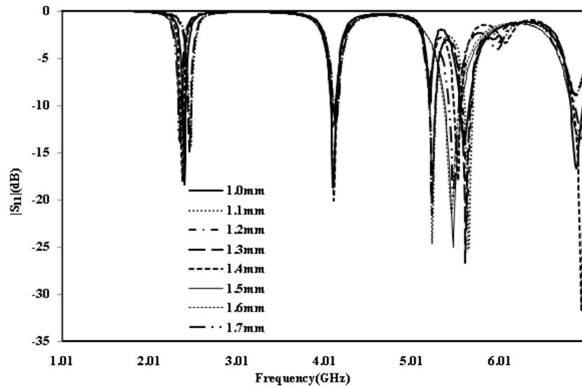
Fig 2: Return loss of antenna for variation in slot
