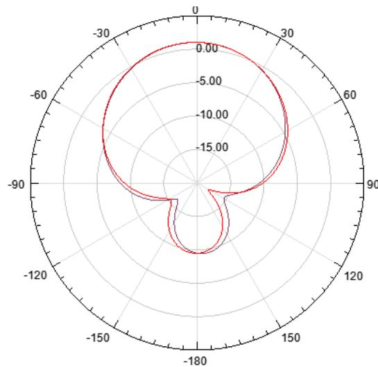
**Fig. 5 Radiation pattern at 3.9GHz**
