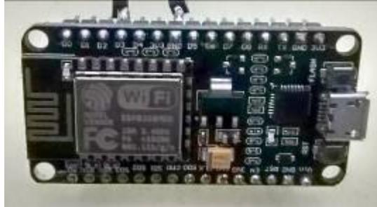
Figure 2: Node MCU ESP8266
