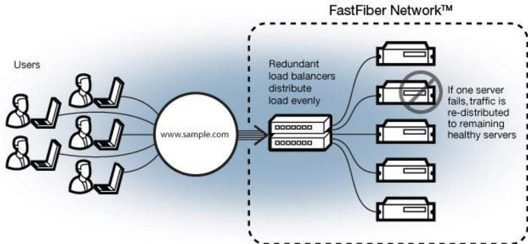
Fig 2: Load balancing in cloud Computing. Load Balancers also help to redistribute the load of a failed node.
