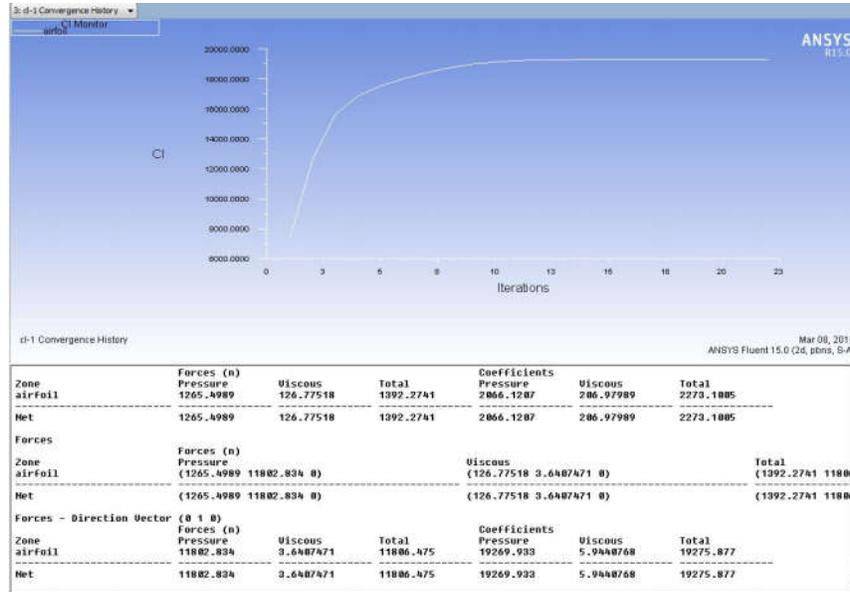
Figure 5. Coefficient of Lift vs Iteration graph
