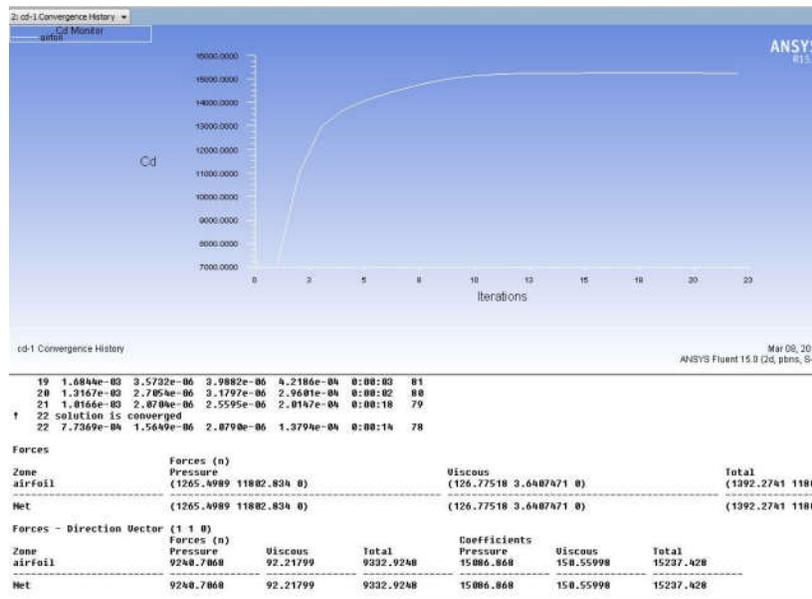
Figure 4. Coefficient of drag vs Iteration graph
