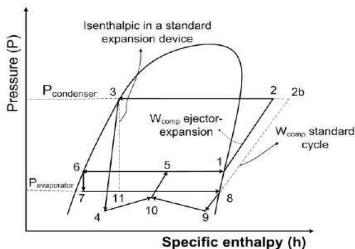
Fig 4. 3: Pressure -Enthalpy diagram of Standard cycle and EERS
