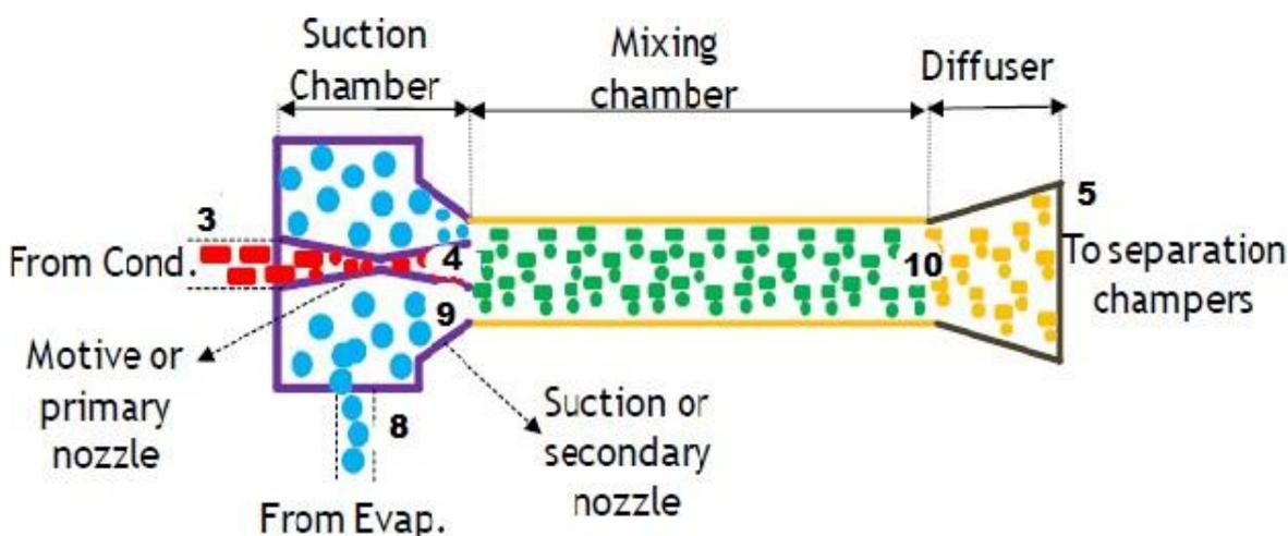
Fig 4. 7: Schematic diagram of flow inside ejector.
