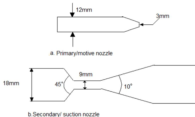
Fig 5: 1 dimension of ejector
