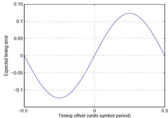
**Figure 2.1. Theoretical S-curve of the Gardner TED for binary PAM**
