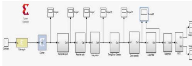
Figure 5.1. BPSK Modem System
