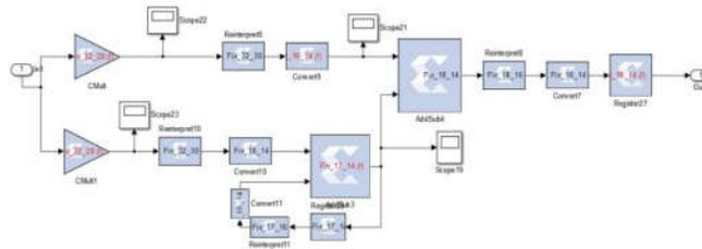
Figure 4.3. Digital Loop Filter
