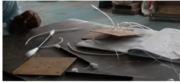
Figure 2: Arrangement of plastic optical fibres in mould
