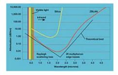
Attenuation in fiber optics, also known as transmission loss, is the reduction in intensity of the light beam (or signal) as it travels through the transmission medium. Attenuation coefficients in fiber optics usually use units of dB/km through the medium due to the relatively high quality of transparency of modern optical transmission media. The medium is usually a fiber of silica glass that confines the incident light beam to the inside.
