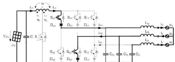
(b) S<sub>a1</sub> ON, S and S<sub>c1</sub> OFF
