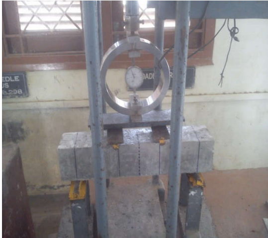
Fig 3: Universal test setup for flexural
