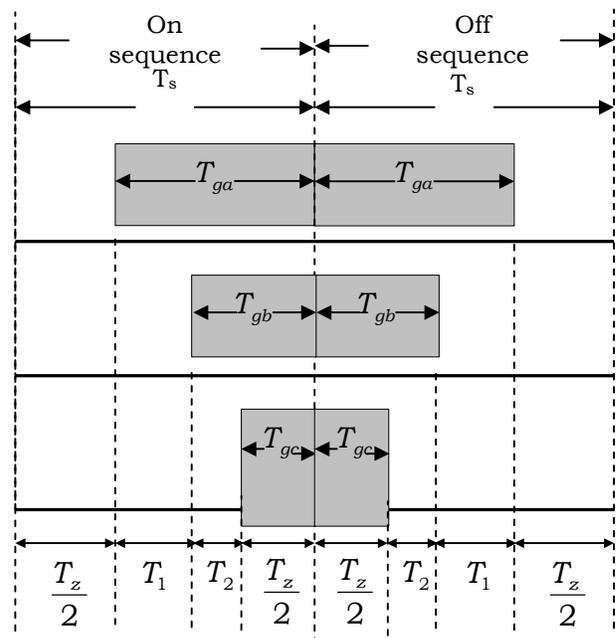
Fig. 2 Gating signal generation using SVPWM scheme in sector-I
