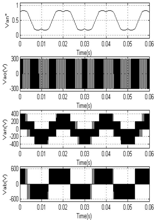
Fig. 3. Simulation results of SVPWM algorithm at modulation index of 0.6
