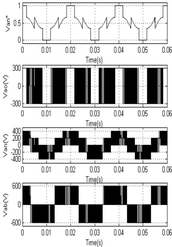
Fig. 7 Simulation results of DPWM1 algorithm at modulation index of 0.6
