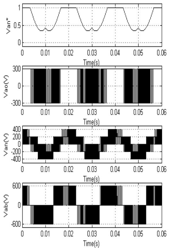
Fig. 5 Simulation results of DPWMMAX algorithm at modulation index of 0.6
