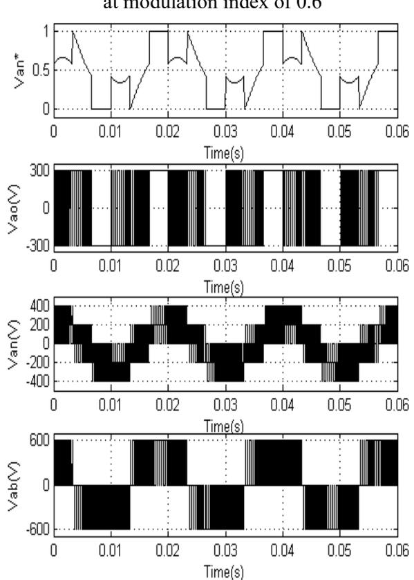
Fig. 6 Simulation results of DPWM0 algorithm at modulation index of 0.6
