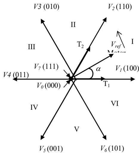
Fig. 1 Possible voltage space vectors and sector definition
