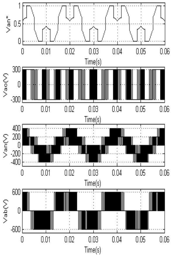
Fig. 9 Simulation results of DPWM3 algorithm at modulation index of 0.6
