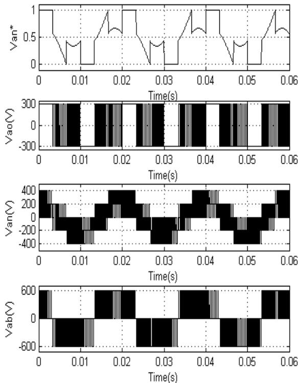
Fig. 8 Simulation results of DPWM2 algorithm at modulation index of 0.6
