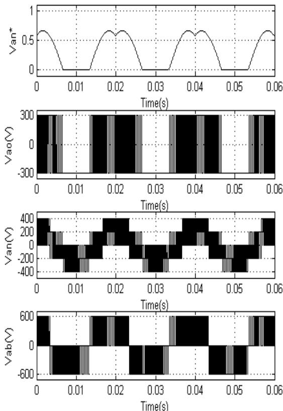
Fig. 4 Simulation results of DPWMMIN algorithm at modulation index of 0.6
