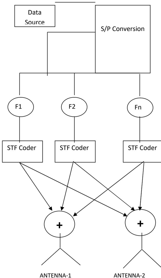
Fig.1. System Model for Separate STF coding rule
