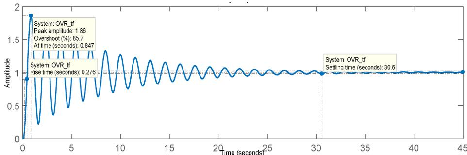
Fig.6. Step output of servomotor without PID controller
