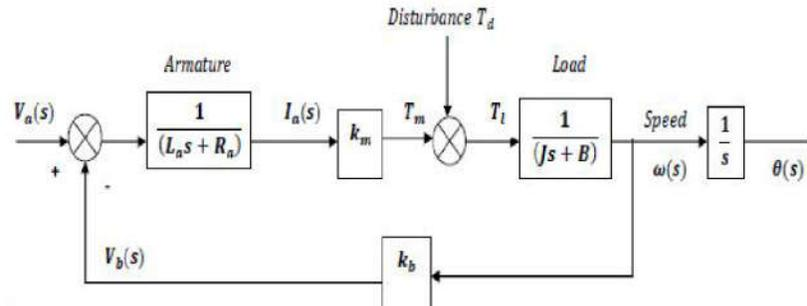
Fig.1. Equivalent block diagram of a pitch-controlling servomotor [2]
