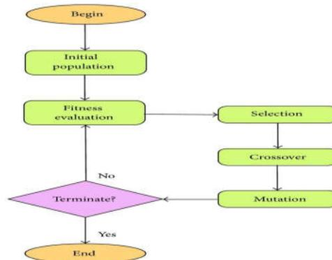
Fig.4 Flow Chart for Genetic Algorithm
