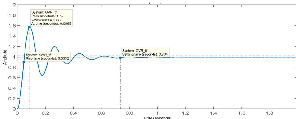
Fig.8. Step response of PSO-PID tuned servomotor
