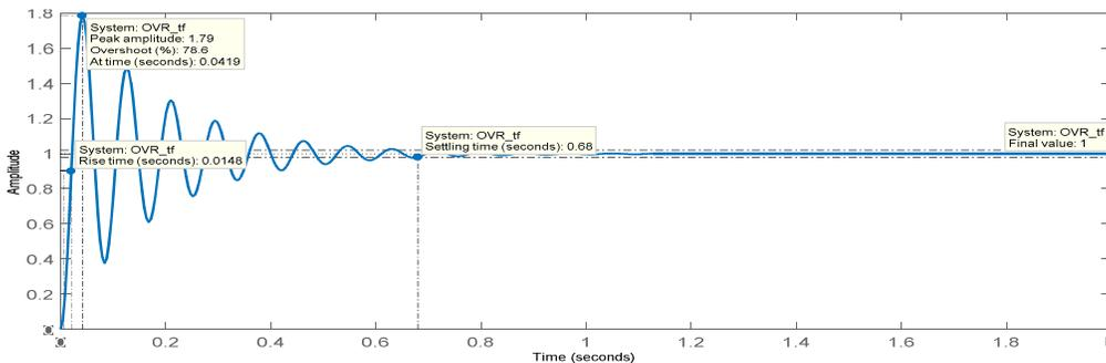
Fig 7. Step Response of GA-PID Tuned Servomotor
