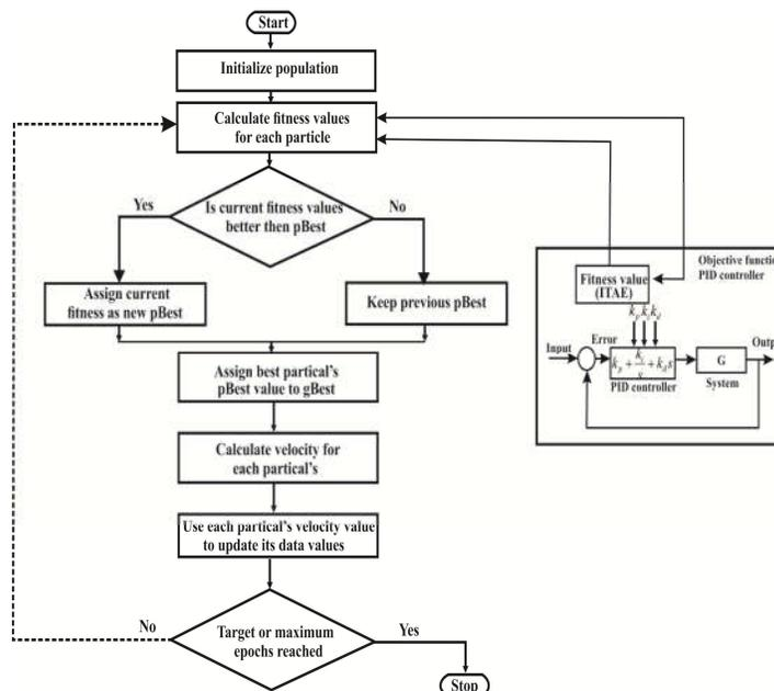
Fig.3. Flowchart of parameter optimizing procedure using PSO [10]
