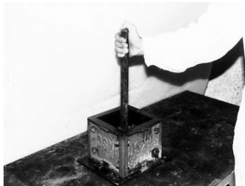
Filling the mould and Compacting the concrete in the cube mould
