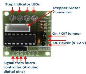
Fig.3 ULN2003A Stepper Motor Drive
