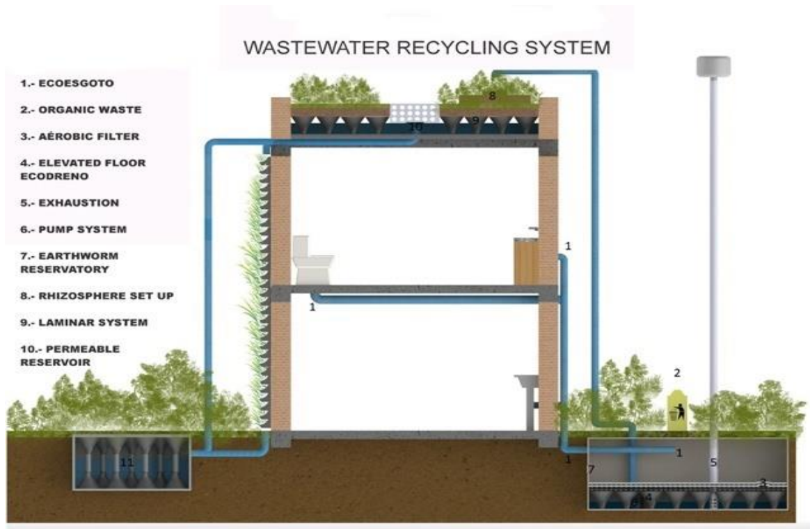
Fig 4: Waste Water Recycling System
