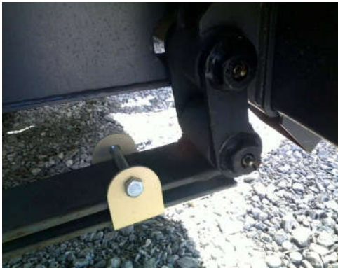
Figure 1.2. Spring with the clamp installed. (Normet Group, Marketing databank)
