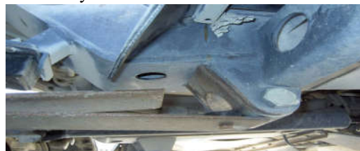
Figure 1.1. Broken spring in the front axle. (Normal Group)
