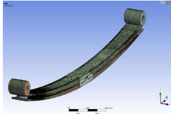
Figure 9.3: Default ANSYS volume Mesh
