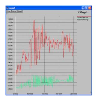
In the below graph X-axis represents time and Y-axis represents the throughput. The Red line indicates the graph for Existing throughput, and Green line indicates the throughput for the Delay responsive protocol. It can be clearly seen that green line is above the red line, indicating proposed throughput it more compared to the existing protocol.
