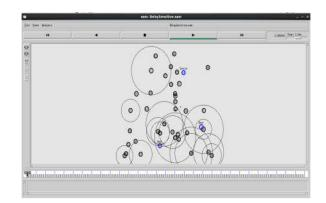
In above screen we can see discovery of neighboring nodes, path discovery and data transmission to destinations via multicast protocol.
