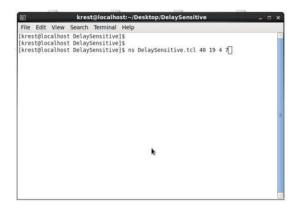
In above screen we are simulating existing MAC layer multicast technique using above command. 40 is total no of nodes and 19 is source node and 4, 7 are destination nodes.
