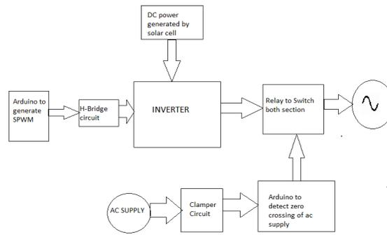
Figure 5: overall block diagram
