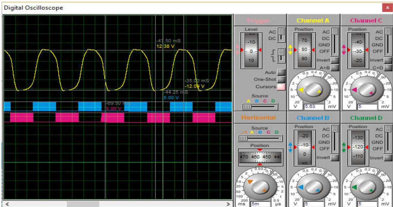
Figure 1: Inverter Output
