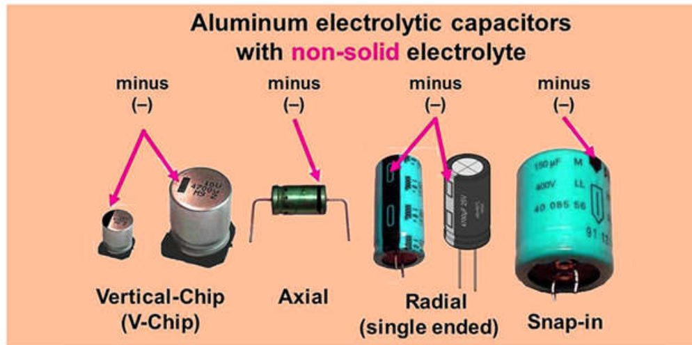
Fig. vii aluminum electrolytic capacitor indicating positive and negative terminals
