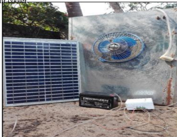
Fig 1.1 FABRICATION ASSEMBLY OF SOLAR AIR COOLER
