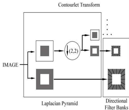
Figure.1 Schematic of Contourlet Transform
