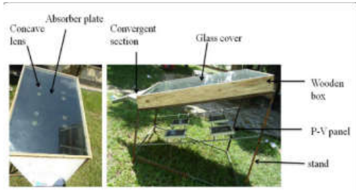
Fig. 4. Final assembly of solar air heater
