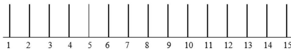
Fig. 2: Spectrum of the FH/CDMA system using 15 frequencies and 15 simultaneous users.
