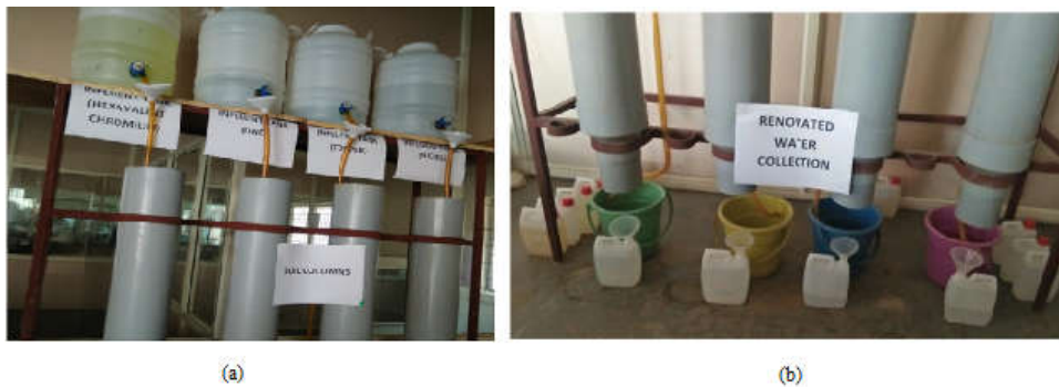
Figure 4. Photographic view of wastewater (a) feeding arrangement and (b) effluent collection system
