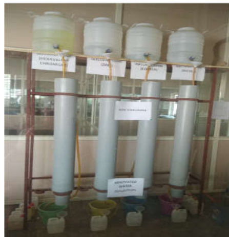
Figure 2. Soil aquifer treatment (SAT) system experimental setup
