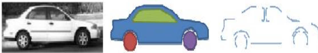
(a) Example image (b) Contour (shape) as feature (c) Contour fragments as feature
